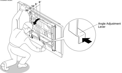
Fix the Angle Adjustment Lever.Once the plasma display has been set at the desired angle, fasten the Angle Adjustment Lever with the screw
